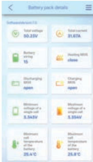
Figure 8: Battery pack details
