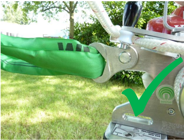
Fig. 7: Correct fastening the EDER Powerwinch 500
