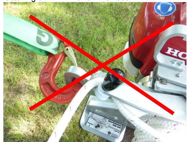
Fig. 6: wrong fastening the EDER Powerwinch 500
